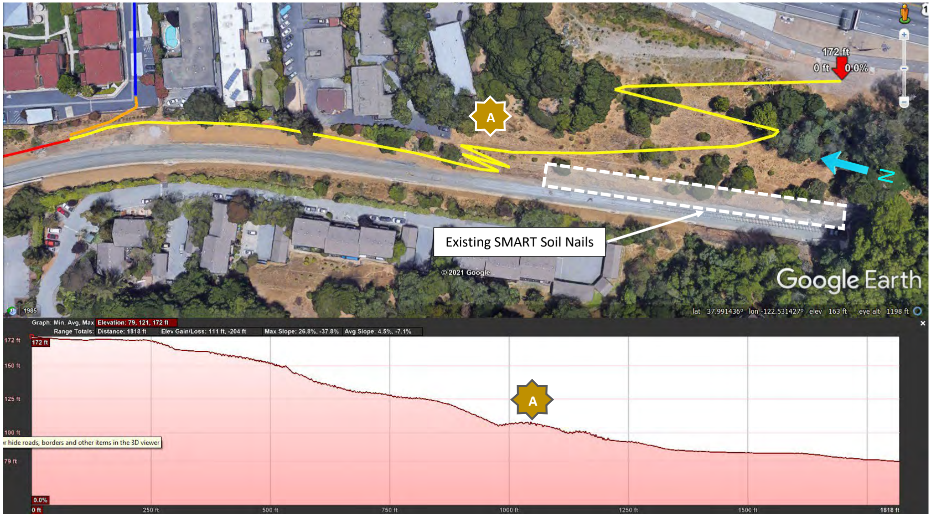
Exhibit 33 - Plan and Profile - Grade to Slope no Greater Than 5% - Location A Highlights Four-Switchback Area
