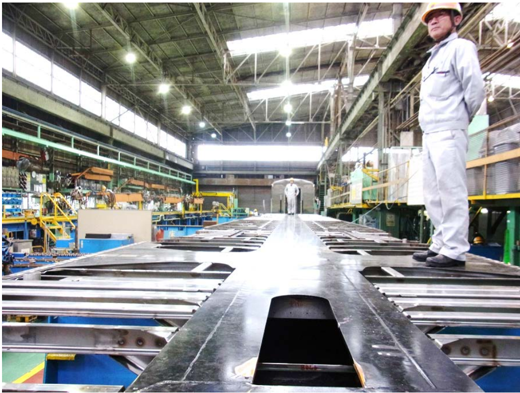
Car No.116 underframe dimension check
